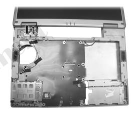
Figure 2-16 Remove the seven screws
